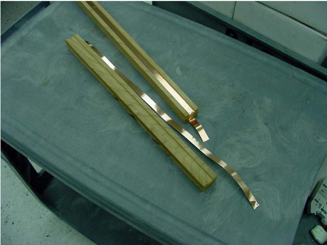
1.  $\frac{1}{2}$ "x  $1\frac{1}{4}$ " harwood was routed with a groove,  $\frac{1}{2}$ " wide and  $\frac{1}{8}$ " deep. This was then laminated to matching, un-groove to provide stability. Once the glue was dry, the wood was cut into a 30" length and an 18" length. My plan was to have a dual ribbon controller for twice the fun!  $\frac{1}{2}$ " wide copper tape was pressed into the groove to provide a conducting point for the resistive element.
