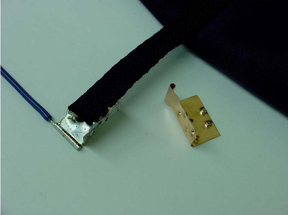
**3.** I made some simple clamps to terminate the resistive element with a wire. This was done with thin copper sheet, punched with a nail for clamping teeth and bent with a small sleeve to hold the 18 awg wire. While soldering the wire into place, I tinned the whole piece of copper. After it cooled, it was pressed around the webbing.
