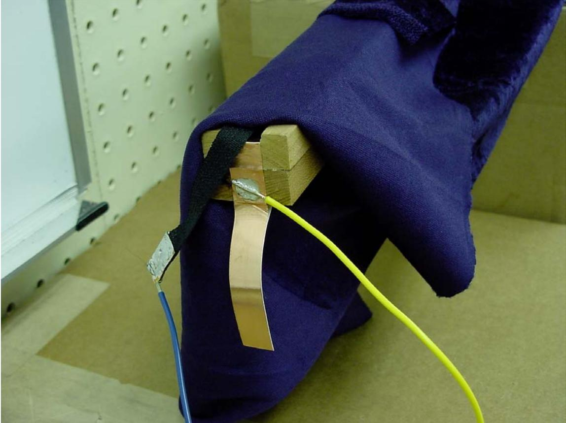
**5.** Here are the two wire connections for the variable resistor assembly portion of the ribbon controller. Now I've got to figure out a good way to attach the velvet to the wood (probably contact cement) and then design a cool-looking casing to hold the two ribbon elements and their associated electronics.
