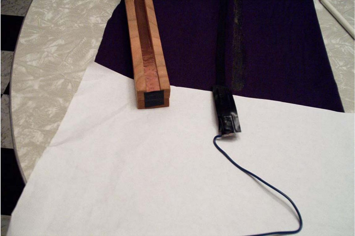
2. While waiting for the cement to set-up, I prepared the terminal ends with PVC tape to insulate them from each other. The corner edges of the copper tape were likewise covered. I felt that if there was going to be a problem area with the webbing contacting the copper tape, it would be here.
