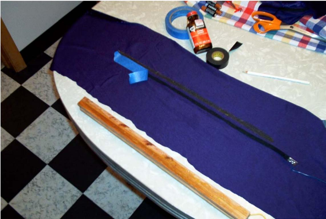
1. After determining the amount of stretch to be applied to each side of the webbing—about an 1/8”—the area that was to be cemented to the wood was coated with the contact cement. I used masking tape to prevent any errant cement from landing on the webbing and to create a nice straight edge for the cement. This would make lining up the wood a cinch.
