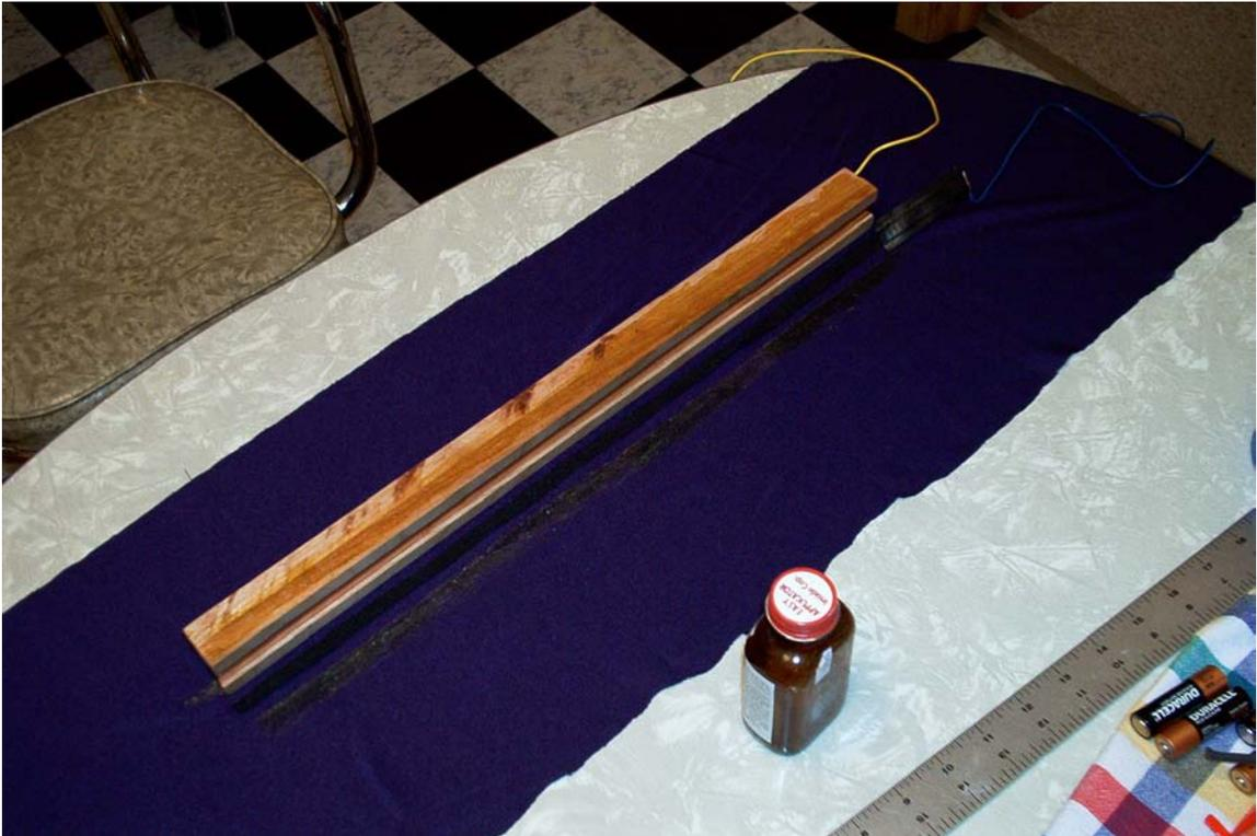
3. Now the surfaces are mated. I lined up the top-corner edge of the wood to the straight edge of the glue. When I was satisfied with the alignment (after what seemed like an hour!), I rolled the wood down onto the velvet and pressed the cemented surfaces together. As you can see in the photo, the next pair of surfaces to be mated were then prepared in the same fashion as the first and with equal care.
