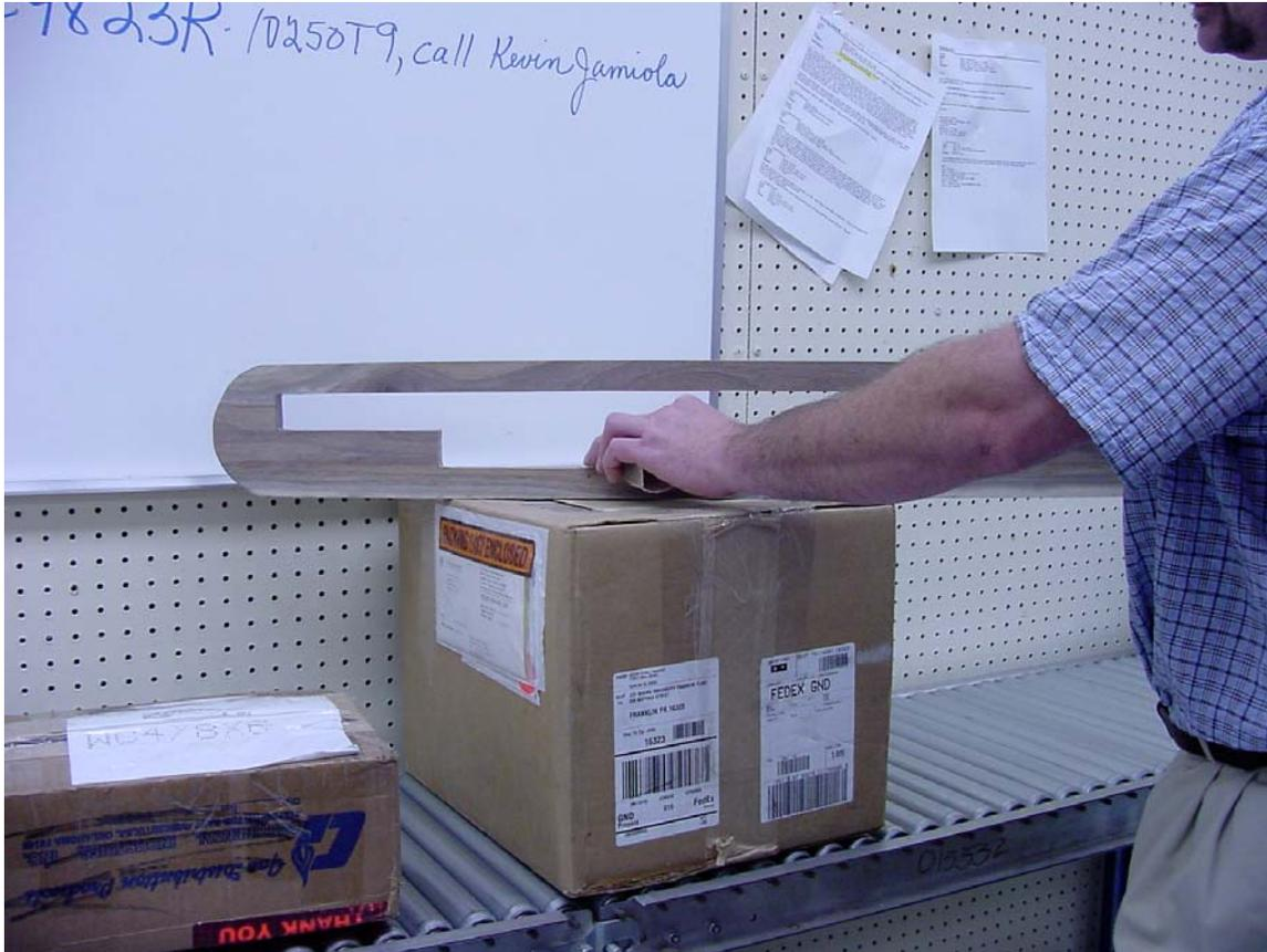
5. Before gluing, the inside cut outs get some final shaping. First with a rough file, then with coarse sandpaper-usually 60 or 80 grit-wrapped around a sanding block. Hand sanding with a block is an efficient tool-watch your work closely.
