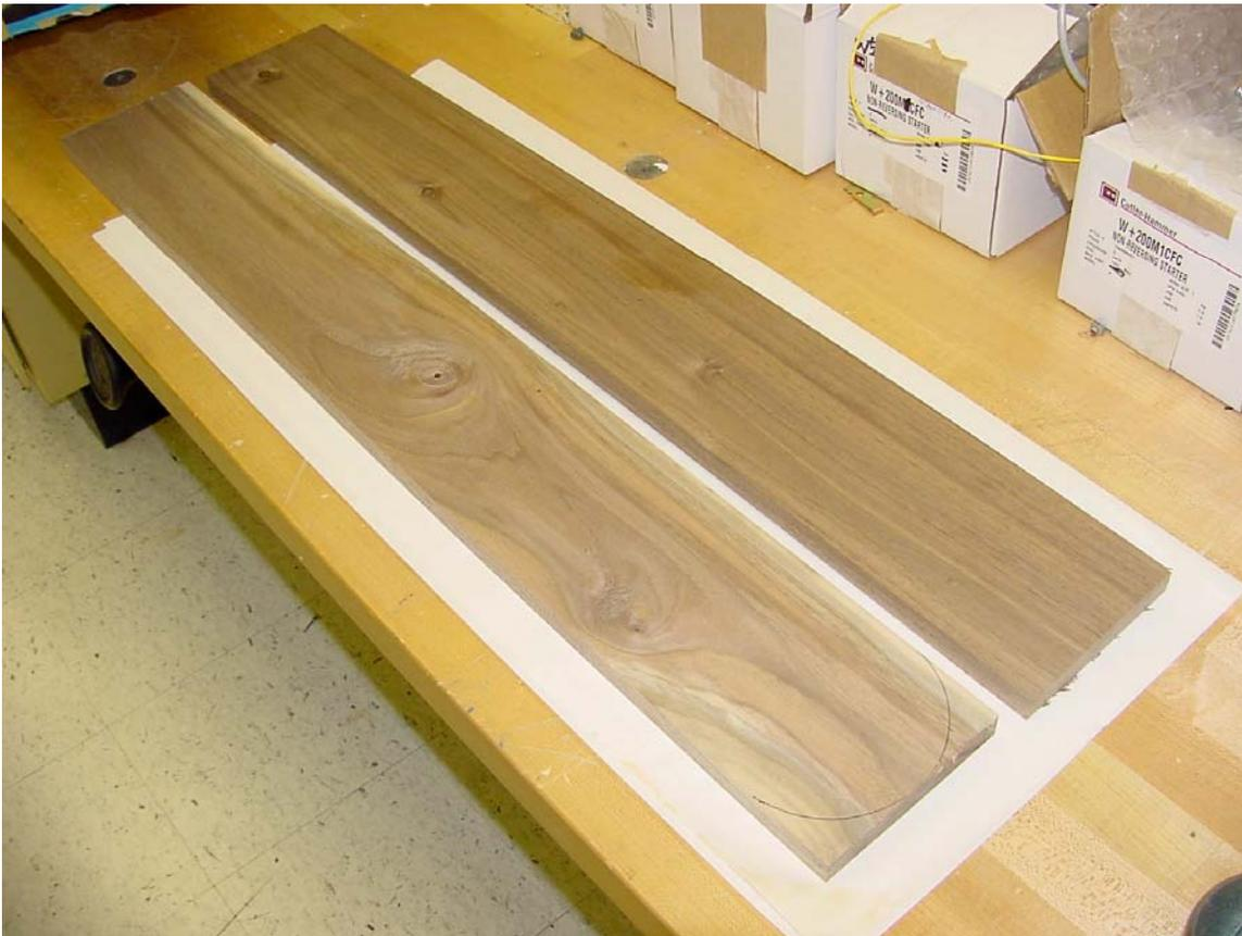
1. Pick your boards and cut to size. These were board ends that my dad cut from the stock still drying in the barn. After planing to  $\frac{3}{4}$ " thickness, the boards were ripped to a 5" width and crosscut to a 36" length. You'll notice that these have some knots-big deal! Look at the color and grain! This is going to be a fun piece.
