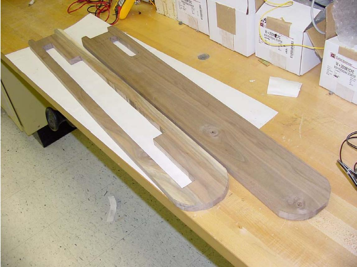
3. Here, the boards are shown after all the rough cutting was finished. There is lots of room for improvement! The board on the right is the bottom. It has a cutout for the electronics. Also notice the ends of both boards. One is radiused and the other end has a cutout for the jack/switch plate to be mounted on that end. Now it's time for the tricky stuff...
