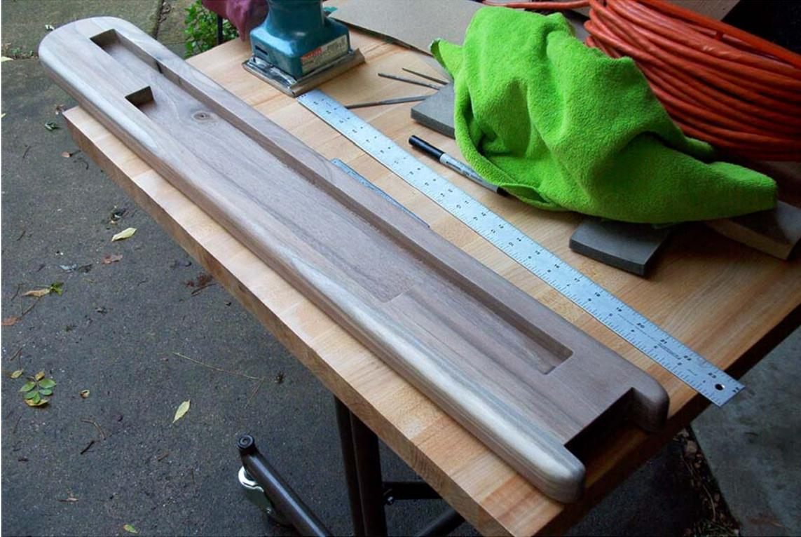
8. It took a couple of hours, but I got the finish sanding finished. For the flat surfaces, I used a random-orbital pad sander. The edges were done with sanding sponges and sandpaper wrapped around a block. The sanding is done when the wood is glass-smooth and you're working with 240 grit paper. My dad said, "just keep sanding 'til you get to 220!" I'm hoping he meant 220 grit and not 220 pounds...
